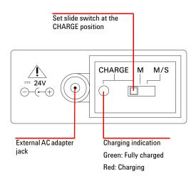
Charge the batteries immediately when the low battery annunciator starts flashing. It is strongly recommended that you use only the specified type of 24 V AC adapter to charge these rechargeable batteries.
